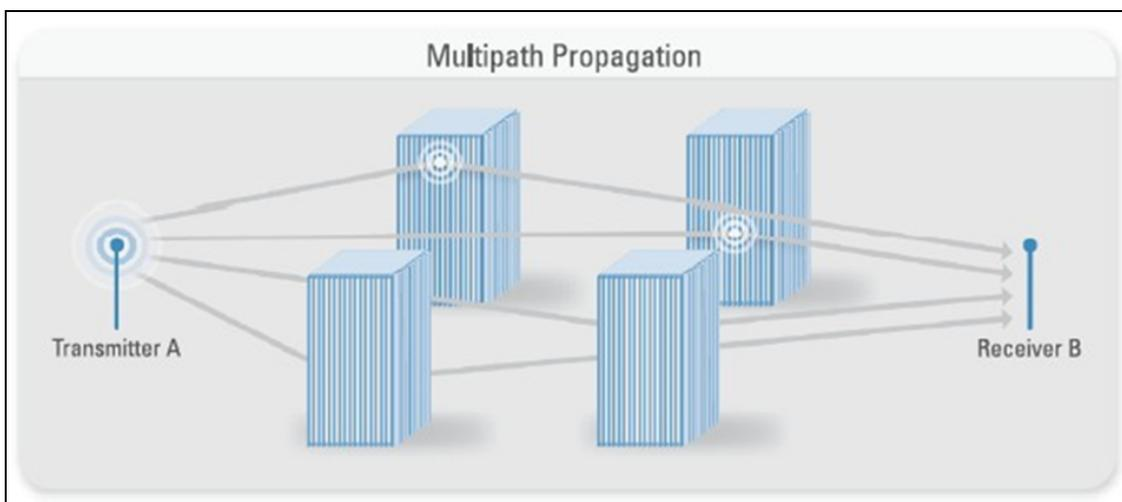
**Figure 2: Multipath Propagation**
