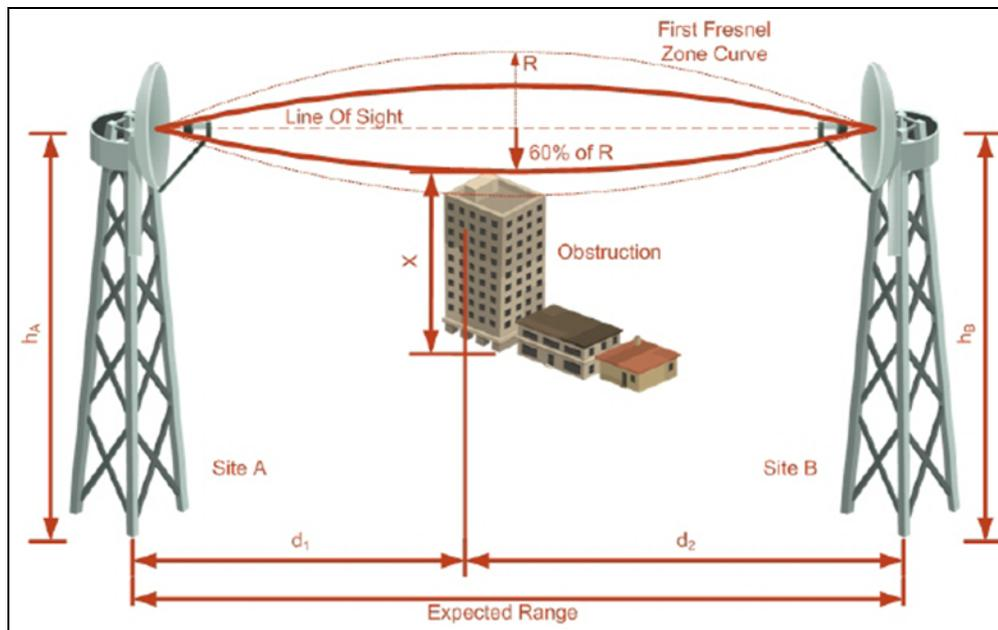
**Figure 1: Encroachment of the Fresnel Zone by a Building**
