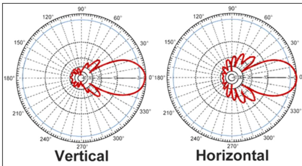
Figure 4: Directional Antenna Radiation Pattern
