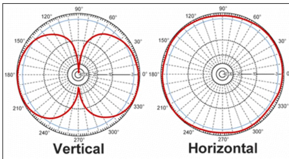
Figure 3: Omni Directional Antenna Radiation Pattern
